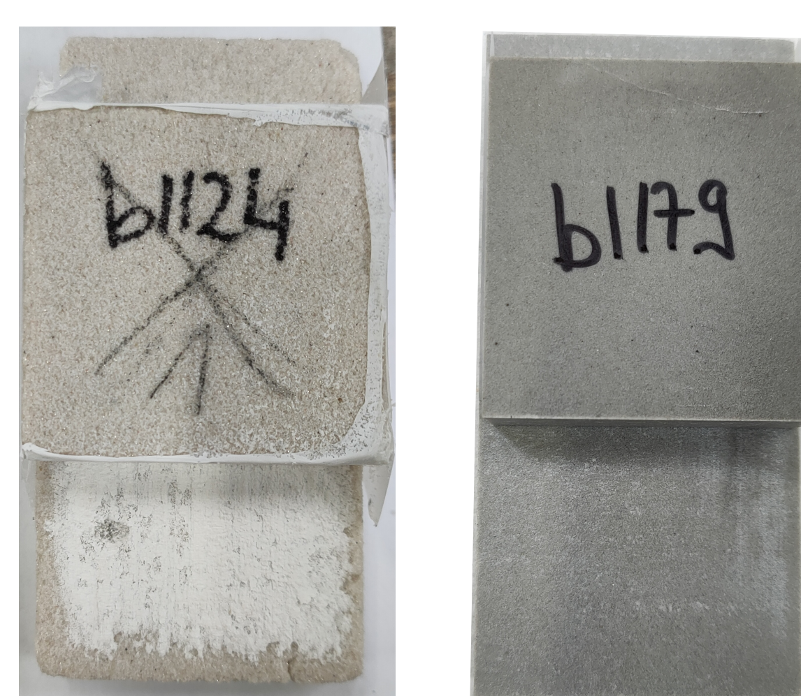
Figure 7: Post-mortem photograph of Fontainebleau sandstone (left) and quartzite (right).
